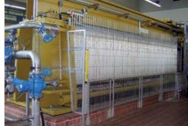
Chamber filter press with feed supply line, NP 150 / NP 40, max. 3 MPa (435 psi)
