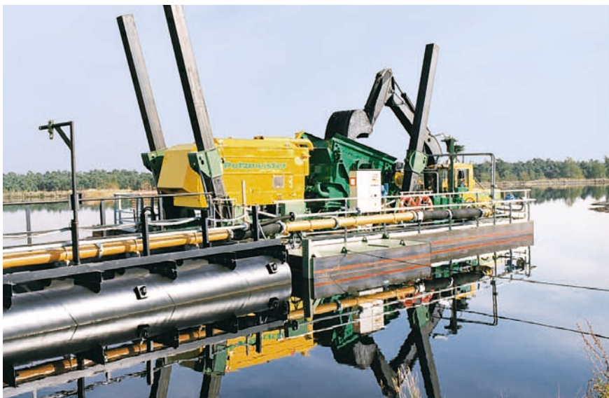
The video cameras and the automatic control system allow remote control from the shore
