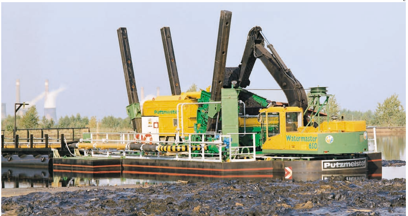
A complete unit – the dredgemaster, consisting of the floating dredge and a KOS 2180 high-density solids pump
