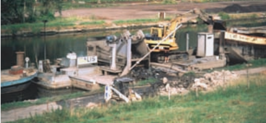
Sludge-processing unit with S-tube pump and hydraulic power pack powered by a diesel motor and fitted to a pontoon in a canal in Belgium
