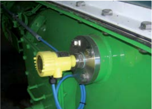
Pressure measurement in the pre-compression zone for optimised regulation of the precompression screw conveyor
