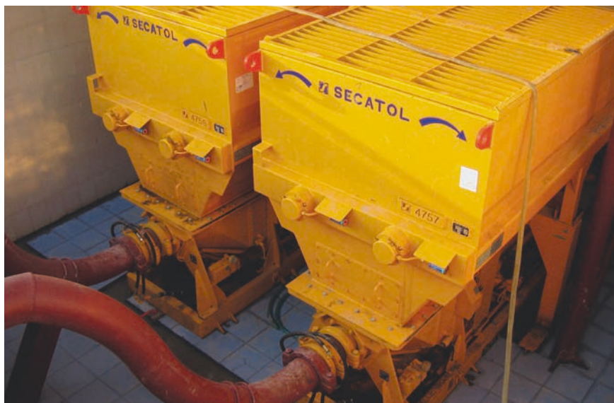
Two S-tube pumps with integral Secatol inlet and mixing hoppers with a volumetric capacity of approx. 7m 3
