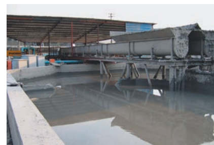
A digger fills the supply screw conveyors with sedimented sludge
