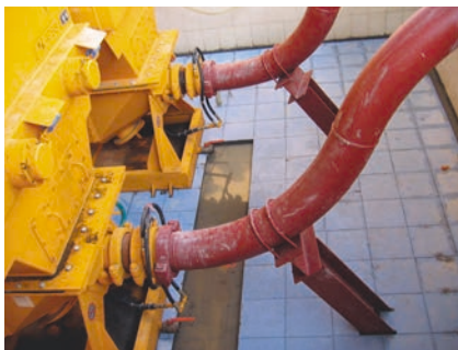
BLI concentric nozzle with water connection for reducing pressure losses
