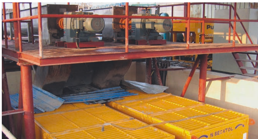
Two S-tube pumps with integral Secatol inlet and mixing hoppers with a volumetric capacity of approx. 7m 3
