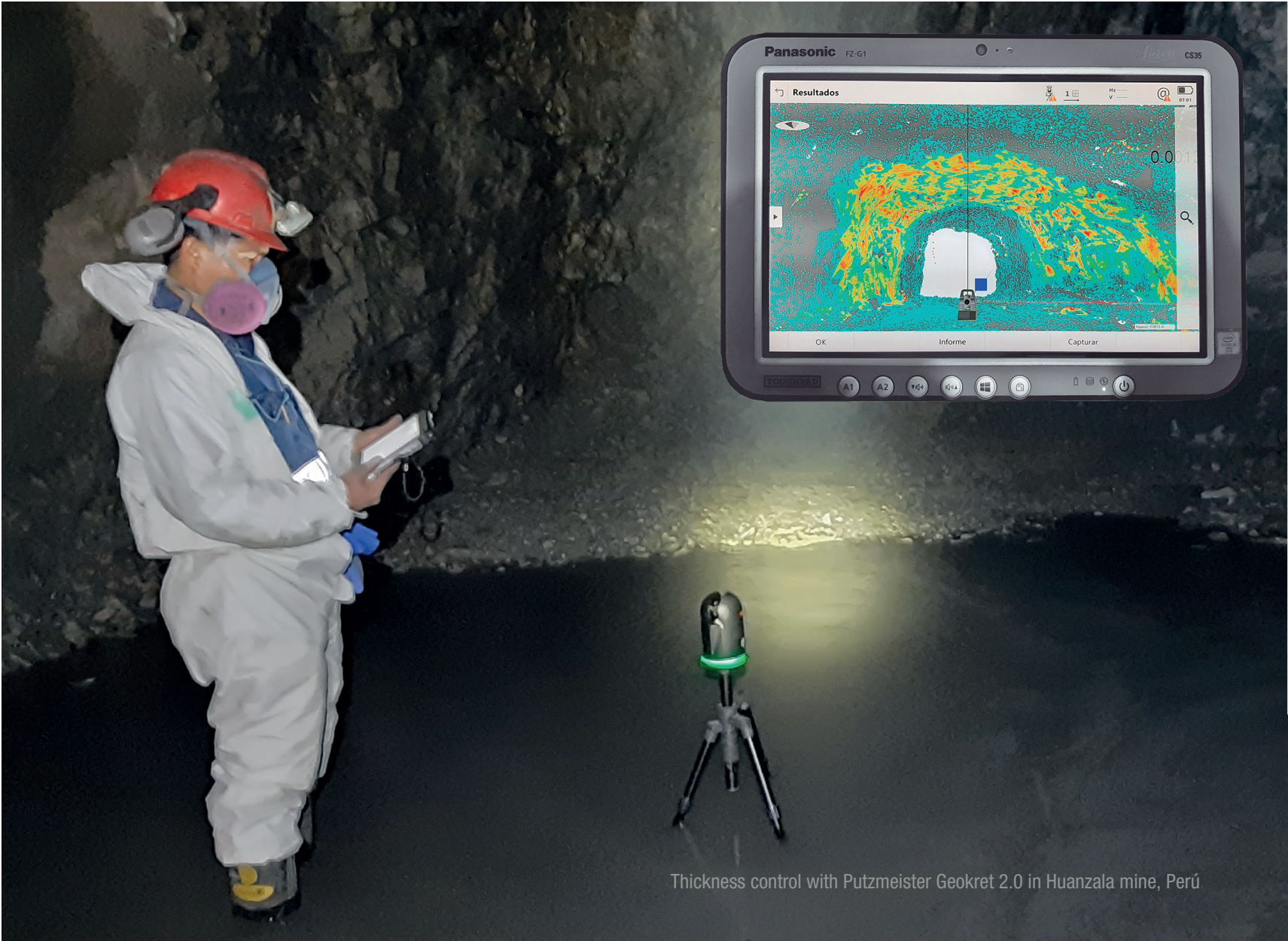
Before (2022): Thickness testing with cores / Now (2023): Testing with Geokret 2.0
