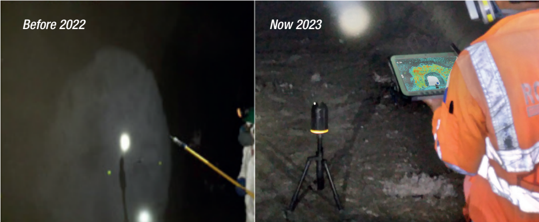
Before (2022): Thickness testing with cores / Now (2023): Testing with Geokret 2.0
