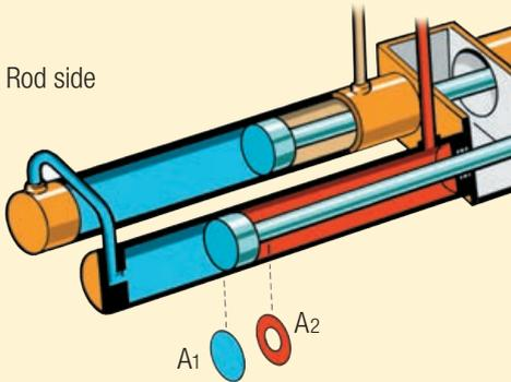
Rod side = lower concrete pressure,
