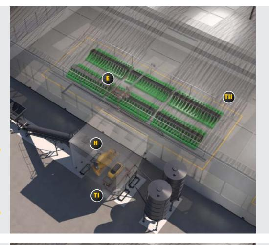
Precise placement of concrete into the battery formwork
