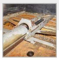
PDL rectangular discharge sliding frame
