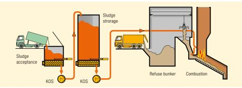
Flow chart: Sewage sludge co-incineration in household incineration plant
