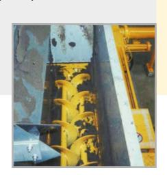
Twin-screw auger feeding device with mixing paddles in the supply chute
