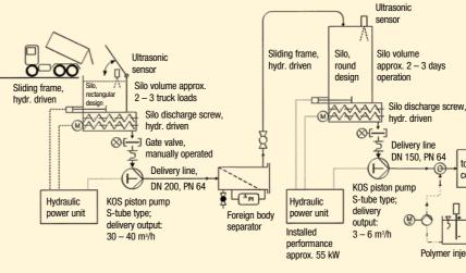
Three types of stations for an efficient sludge handling system
