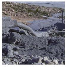
Above: Fly ash hardens within a short time **Right:** A KOS 25100 pump installation (Kogan Creek, Australia) for fly and bottom ash
