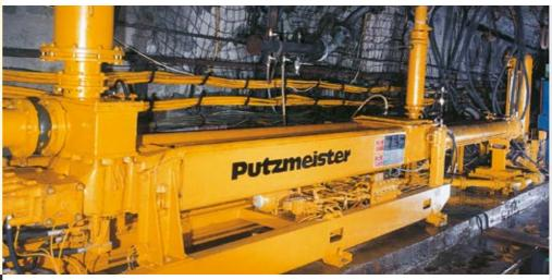
Handling of iron ore concentrate with two HSP 25200 HP in Russia, Staryj Oskol, (distance 26.5 km)
