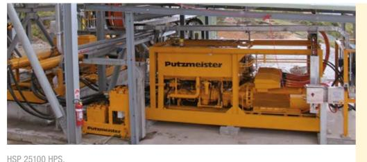
Hydraulic Powerpack PCF Pumping pressure characteristic of an HSP pump with PCF: Pipeline pressure diagram 8 MPa / flow rate 130 m3/h
