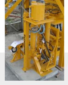
each delivery stroke of the pump. The content of this third cylinder is actively pushed into the delivery pipeline during the changeover of the Piston pump.
