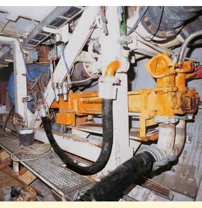
A KOV 1050 pumps the injection mortar behind the ring segment
