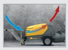
The innovative exhaust air routing and an additional exhaust duct improve the working area.
