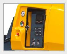
The central operating panel with intuitive keypad employs the "follow the blue light" principle, is easy and safe to operate and is well protected by a robust acrylic-glass door.
