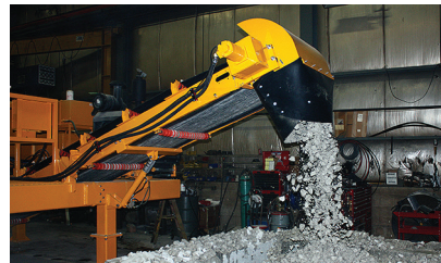
Unique auger flights move material to center of hopper to assist with feeding material to discharge gate. Discharge gate is hydraulically operated and adjustable to match control flow of material on the conveyor. Auger is variable speed, providing maximum control and reduced wear.
