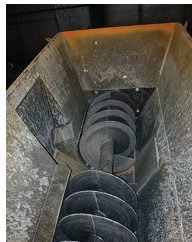
View inside hopper: Bi-directional, variable speed 36" (915mm) diameter auger with hard-faced flights for extended life.
