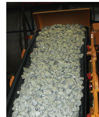
36" (915mm) wide hydraulically operated variable speed conveyor can discharge concrete, RCC, rock, sand or dirt.
