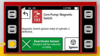
Clearly guided fault management on the radio remote control and the graphic display
