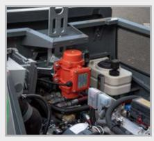
The new "ICC" vibrator is located outside the dirt area under the hood. This is also where the optional battery charger for the wireless remote control with precise delivery rate adjustment can be found.
