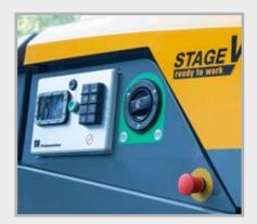
The control panel with an intuitive keypad increases operational safety.
