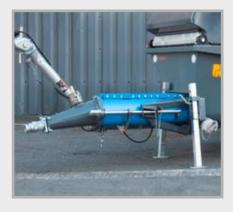
The patented quick-change system for the worm pump saves time and facilitates the handling. Without additional tools only one person is needed to change even the the heaviest 2L8 rotor/stator combination.
