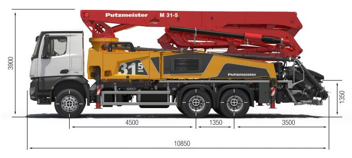
Note: Standard version. Dimensions and weights depend on truck and pump model. Dimensions in mm, MB-Actros 3243 as example. For illustration only.
