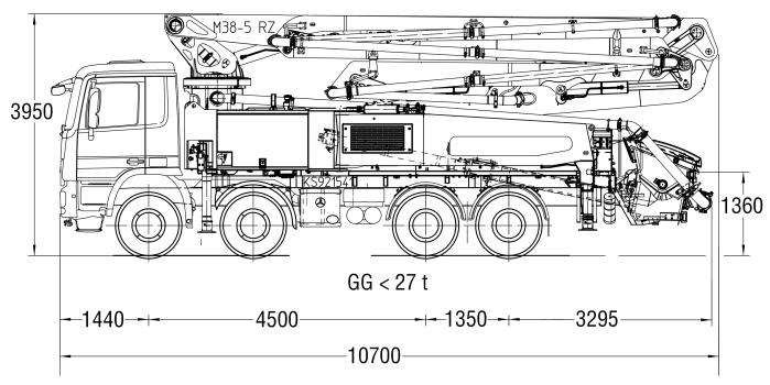
Note: Standard version. Dimensions and weights depend on truck, pump model and equipment. Dimensions in mm for MB-Actros 3241B(3244B)/8x4/45.
