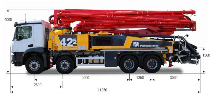
Note: Standard version. Dimensions and weights depend on truck, pump model and equipment. Dimensions in mm, MB Arocs 3240.
