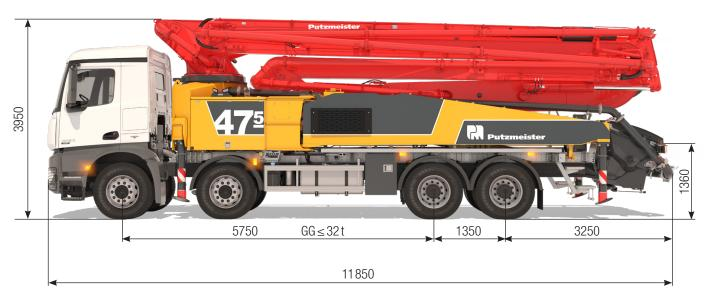
Note: Standard version. Dimensions and weights depend on truck, pump model and equipment. Dimensions in mm, MB-Arocs 4143 as example. For illustration only.
