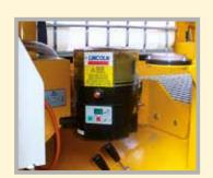
Centralized lubrication system for proper machine maintenance
