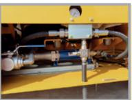
Screw additive pump with flowmeter to ensure a high-quality finish
