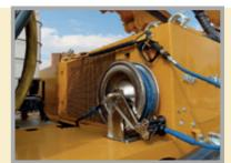
Built-in cleaning system with diesel and electric operation
