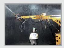
Optional Hydroscaling system for surface cleaning
