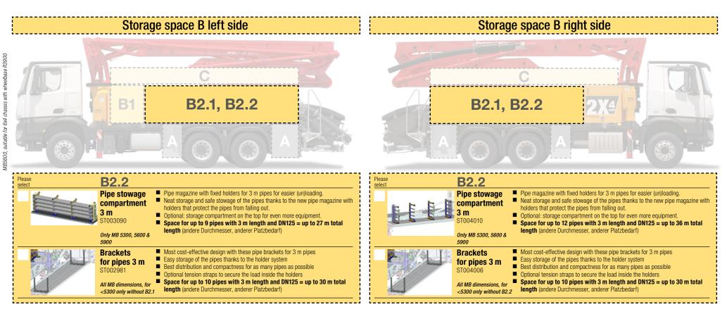
MB5600, suitable for 6x4 chassis with wheelbase R3900
