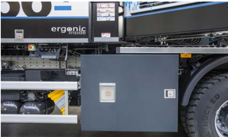
Switch cabinet with main switch
