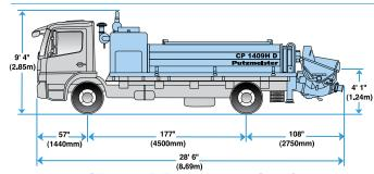
CP 1409H D Truck-Mounted Specifications Based on Model MB Ateon 1318. Shins without truck Chassis shown is an example
