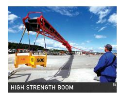
Four-section boom retracts to 74' 9" (22.80m), providing an expansive working range. Infinitely variable belt speed control through radio remote offers smooth and controlled movement. The advanced boom design with modern lattice structure made of extruded steel tubes is extremely strong, yet lightweight.
