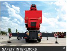
Safety is engineered into the TB 200, with multiple safety interlocks that prevent improper operation, including driving the unit with the boom not properly stowed, running the Telebelt when outriggers are not fully deployed, and operating the Telebelt with an incorrect counterweight position.
