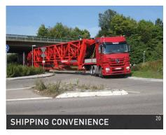
Able to be shipped globally for any project, the TB 200 is transported in the following four main components: the chassis — which can be self driven and shipped RO/RO, the boom and feeder package — which is shipped break bulk, and two ocean containers — one for the counterweight and one for the work platforms, feeder slewing gear and ancillary items.
