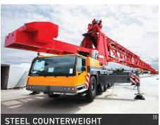
The TB 200's steel counterweight is a structural component of the unit. The counterweight moves proportionally in and out as the boom extends and retracts, ensuring that the right amount of weight is in the right position to offset the load of the boom. Its lighter counterweight requirement decreases the weight on each axle, providing greater efficiency.
