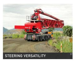
Steering of the TB 200 has been engineered to provide a tight turning radius for necessary job site maneuverability. It features all-wheel steer, eight wheel drive, and a self-leveling chassis. Steering modes are: on-road, all-wheel, crab steer, reduced sheer, and independent rear axle mode.
