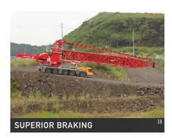
Recognizing the importance of being able to safely stop heavy machinery, especially in rough conditions, the TB 200's superior braking system offers four types of braking: parking, service, engine, and transmission. Testing demonstrates that the TB 200 can effortlessly handle grades, as well as stop and re-start on them.
