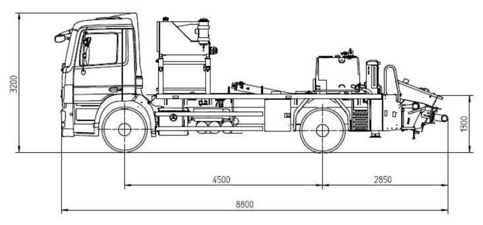
Note: Standard version. Dimensions and weights depend on truck, pump model and equipment. Dimensions in mm. For illustration only.
